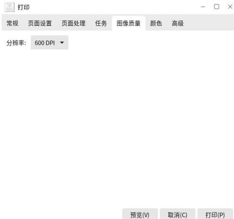
The higher the resolution, the better the printing effect; the lower the resolution, the higher the printing speed.
