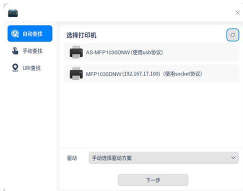
If the network printer cannot be found in the "Select Printer" list, click "Manual Search" and enter the IP address of the printer in the address bar on the right (default IP: 192.167.17.100).
